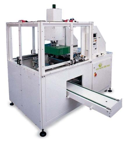
The Endoline 500 series of tray erectors is designed to be flexible enough to produce a wide range of tray sizes and styles at up to 25 trays per minute. They are operator friendly machines that are easy to maintain and extremely simple to operate and adjust.
